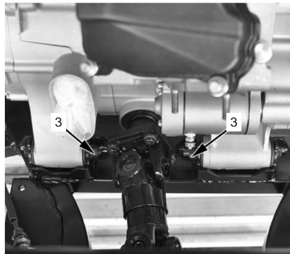
3. Rear engine mount bolts
