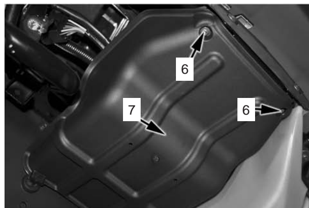
5. Center panel, front 6. Bolt 7. Hood/ dashboard
