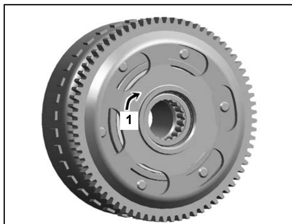
Sprag Clutch Functional Test 1. Lock Direction
